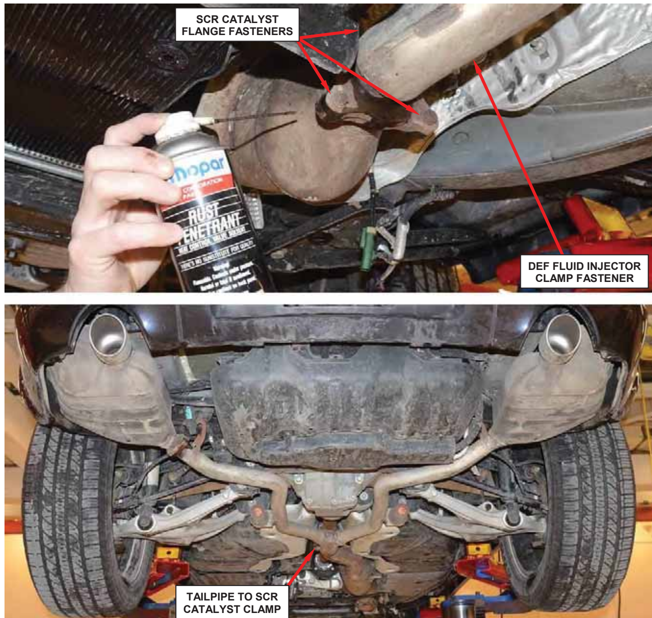
Figure 3 – Saturate Exhaust Fasteners with Penetrating Lubricant
